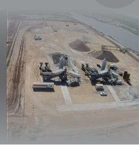
Three LNG Trains (Trains 1 through 3), a Common Gas Pre-Treatment Unit, and a Loading Dock are currently being constructed and connected to the existing facility to complete this turnkey natural gas liquefaction facility now that ground improvement activities are complete. This LNG Facility expects to achieve commercial operation of the first liquefaction train in 2018.
